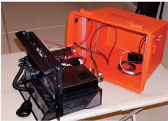
Ready to Assemble Chassis into SPUD-7 Box
