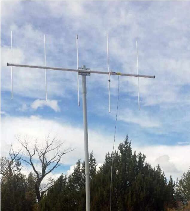
In the mean time, I discovered I had the Yagi mounted in the wrong place and on Monday I was using an aluminum mast (not shown) as opposed to the non-conducting one in the above photo. I moved the mounting plate to the rear of the Yagi and dug out my schedule 80 mast. I was excited, I knew it was going to work better.
