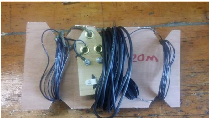
Picture of portable 20m antenna rolled up
