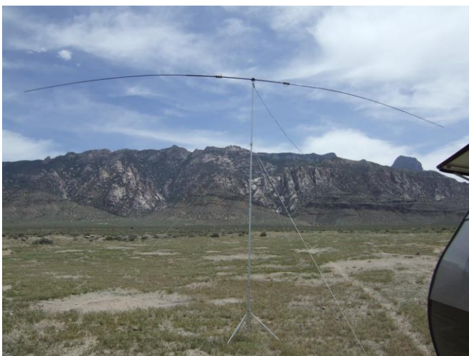
Figure Buddi Pole in a dipole configuration with taps on the coils for quick 20 and 40 meter band changes.
