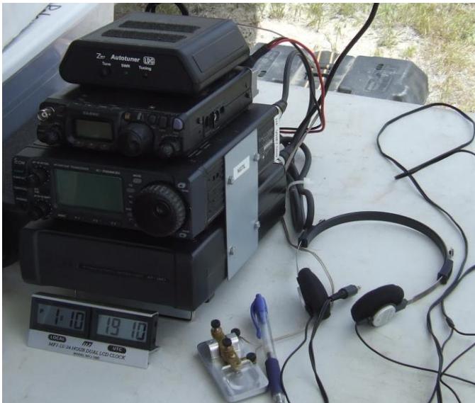
Figure 1 Icom 706MKII with auto tuner, FT817 and tuner for QRP, and a portable lightweight straight key.
